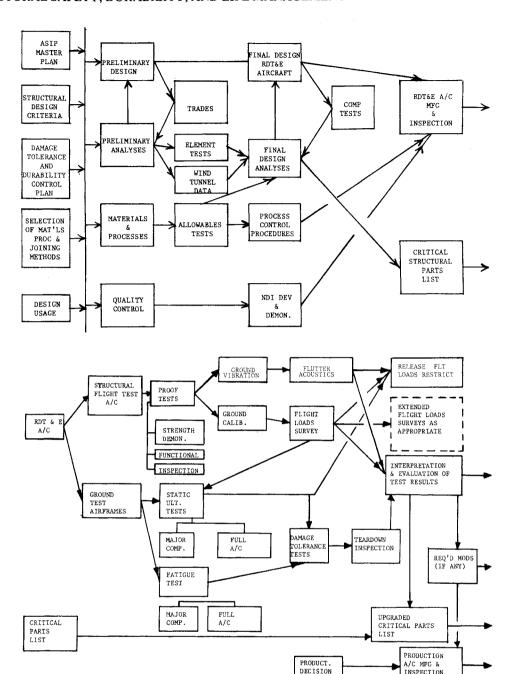
Fig. 2 Design analysis and development tests.
